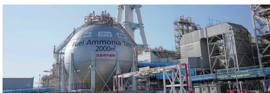
Newly built ammonia fuel tank for large-scale demonstration testing
